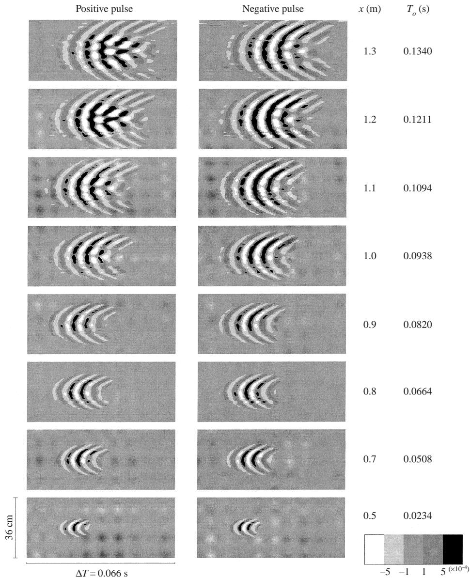
FIGURE 1. Comparison of the evolution of the positive and the negative wavepackets on a time-span plane shown by contour plots of the streamwise velocity fluctuation non-dimensionalized by the free-stream velocity. The measurements were taken at  $y = 0.6\delta^*$ .  $T_o$  is the time delay between the excitation and the beginning of the interval  $\Delta T$ .
