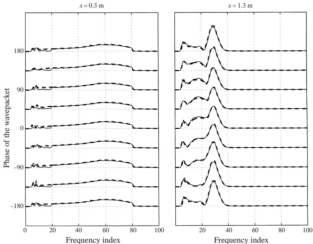
FIGURE 7. Fourier domain. Comparison of the nonlinear wavepackets created with the complete excitation time series (thick dashed lines) and the nonlinear wavepackets created with the truncated excitation time series (thin lines) for different wavepacket phases.
