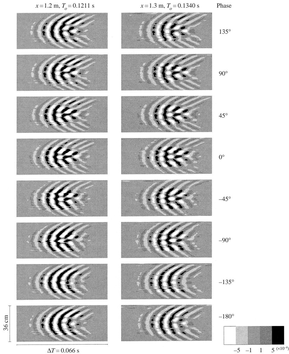
FIGURE 2. Variation of the nonlinear behaviour with the wavepacket phase on a time-span plane shown by contour plots of the streamwise velocity fluctuation non-dimensionalized by the free-stream velocity. The measurements were taken at  $y = 0.6\delta^*$ .
