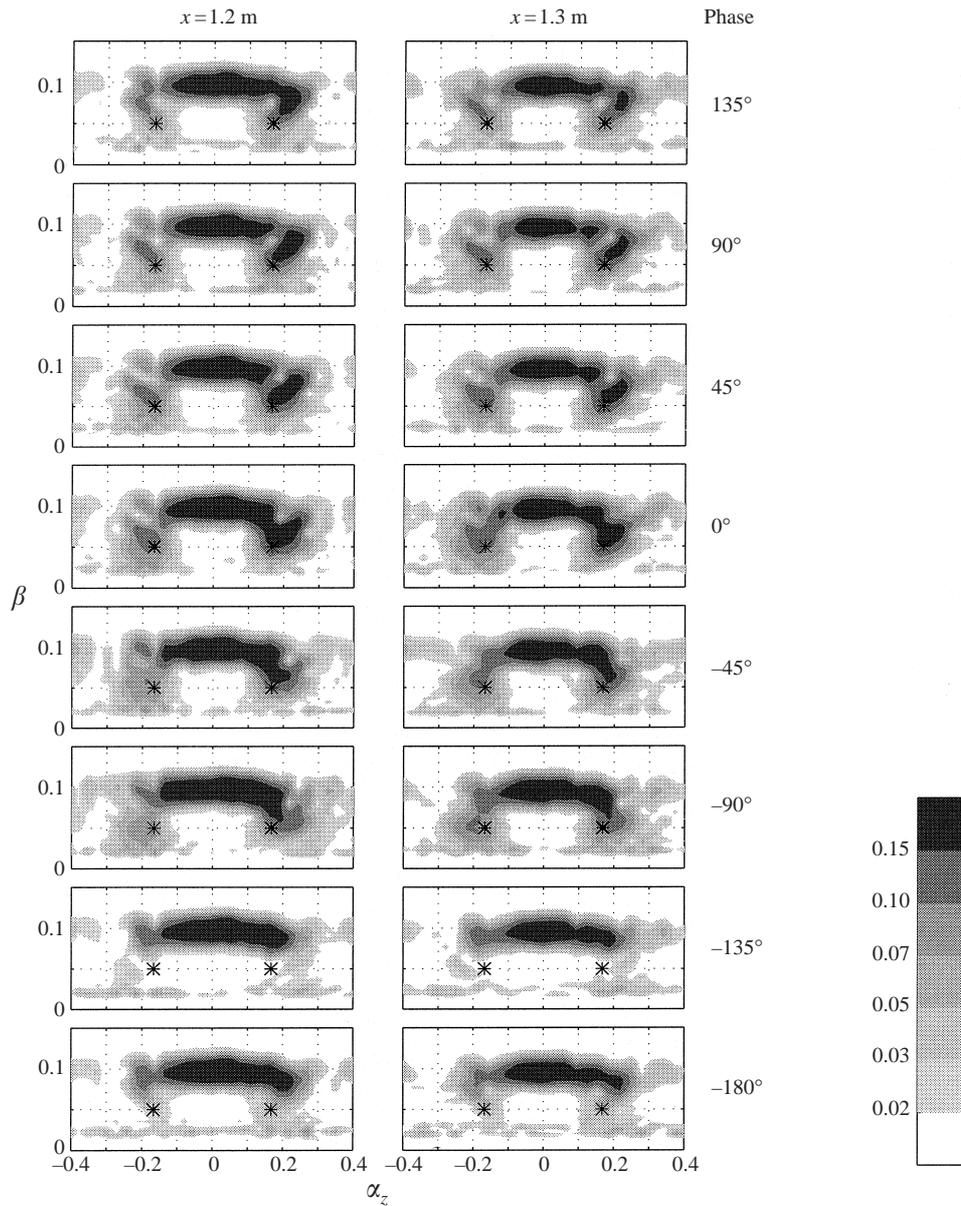
FIGURE 4. Variation of the nonlinear behaviour with the wavepacket phase shown in the frequency ( $\beta$ )  $\times$  spanwise wavenumber ( $\alpha_z$ ) plane. Measurements taken at  $y = 0.6\delta^*$ . The plots show the relative magnitude. The asterisks indicate the waves satisfying Craik's resonance condition.
