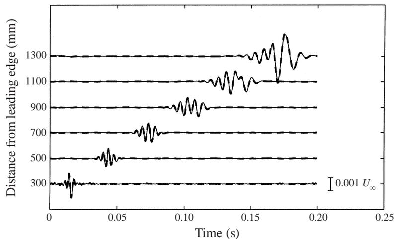
FIGURE 6. Physical domain. Comparison of the evolution of a wavepacket created with the complete excitation time series (thick dashed lines) and a wavepacket created with the truncated excitation time series (thin lines).
