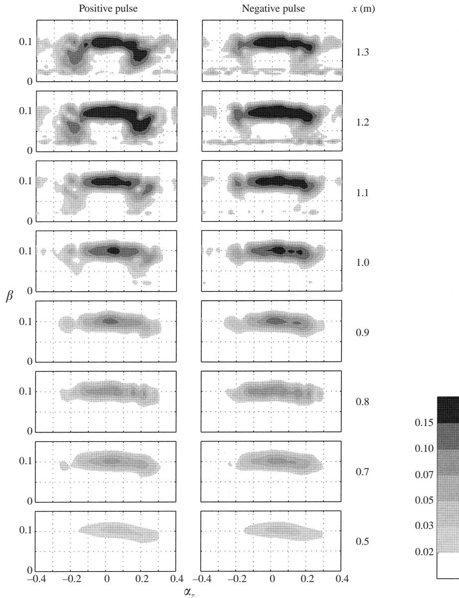
FIGURE 3. Comparison of the evolution of the positive and the negative wavepackets in the frequency ( $\beta = 2\pi f\delta^*/U_\infty$ )  $\times$  spanwise wavenumber ( $\alpha_z = 2\pi\delta^*/\lambda_z$ ) plane, where  $f$  is the dimensional frequency and  $\lambda_z$  is the dimensional spanwise wavelength. The plots show the relative magnitude. Measurements taken at  $y = 0.6\delta^*$ .
